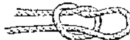
Slip or running knot
